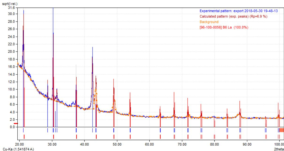
Figure 1 Diffraction pattern from commercial LaB<sub>6</sub>
